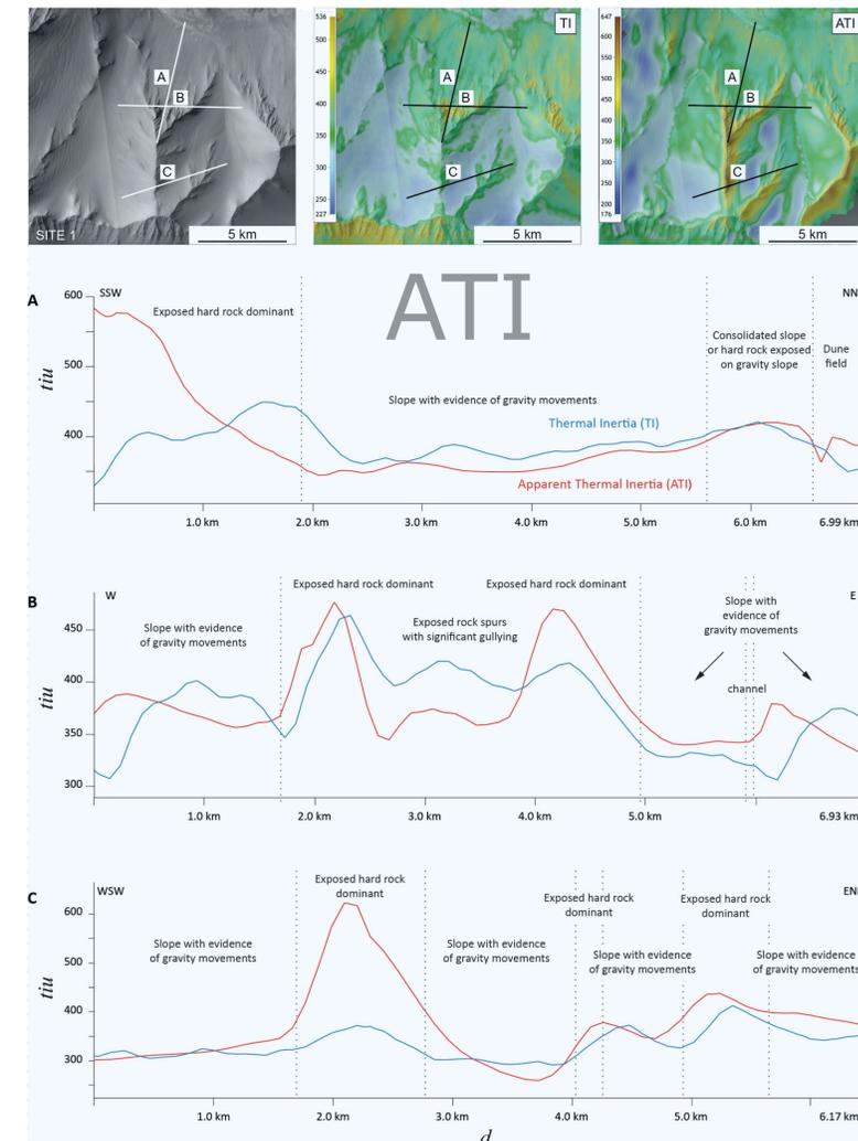
Figure 2. Comparison between TI and ATI (in  $\text{tiu}$ :  $\text{J m}^{-2} \text{K}^{-1} \text{s}^{-1/2}$ ) values obtained on various slopes along profiles A to C. Maps at the bottom: MRO/CTX image; TI map; ATI map. TI and ATIC are overlain onto the MRO/CTX image
